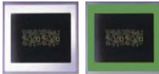
Figure 2. Lead-bearing (l) and lead-free (r) stencils show distinguishing marks to help avoid contamination.
